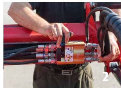
Disconnect the power cable and all hydraulic connections to BX belt with one single lever.
