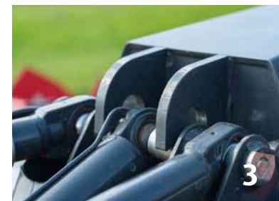
Lower the mowing units and the BX belt automatically comes off.
