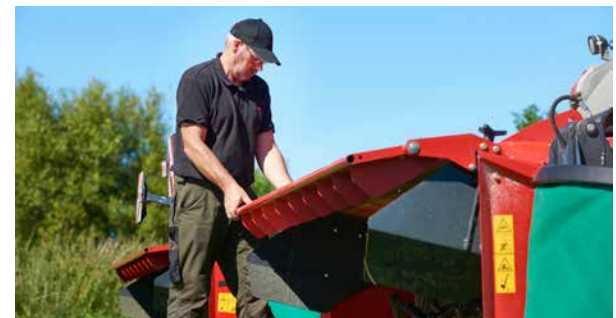
The swath plates are easily slid to the side and the FlipOver widespreading vanes are turned 180°. No tools are required.
