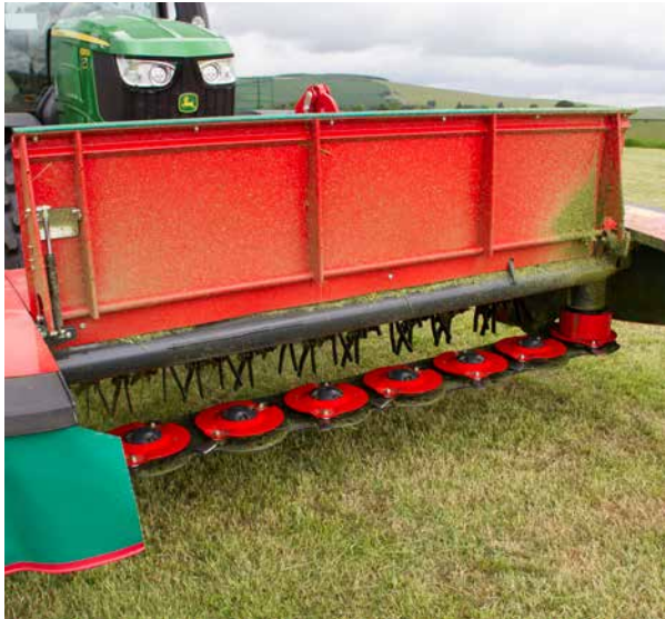
Easy access for inspection and service. The complete front opens to a vertical position via a hydraulic cylinder.
