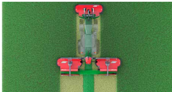
One large swath from up to 9.5m working width.
