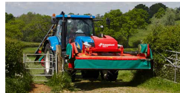
Foldable sideguards ensure narrow transport width.
